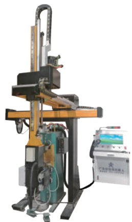
桁架机器人自动焊机 Truss Robot Automatic Welding Machine
